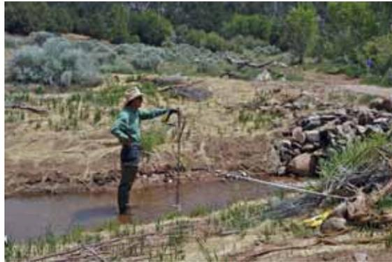
Neil Williams of Watershed West was the project engineer and lead designer for the restoration project. Here, Neil is making a stream discharge measurement to determine how much our river is flowing!
